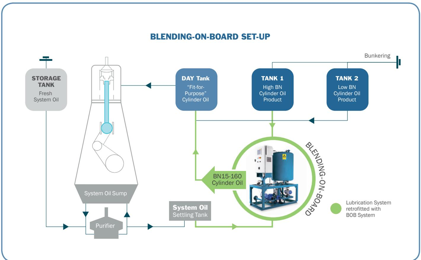
SEA-Mate Blending-On-Board system with an example of pipe layout.
